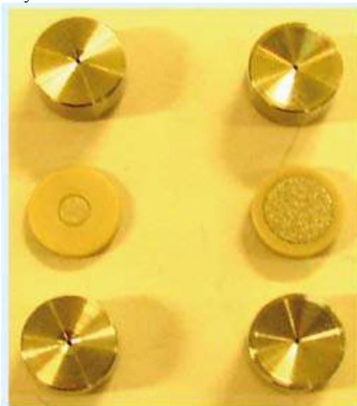
**Figure 9** Protection for 4.6 and 2.1 mm id columns packed with 1.8  $\mu\text{m}$  particles, inlet frit with 0.2  $\mu\text{m}$  pore size.
