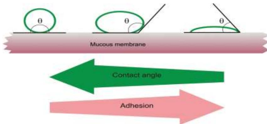
FIGURE 6. Schematic diagram showing influence of contact angle between device and mucous membrane on bioadhesion
