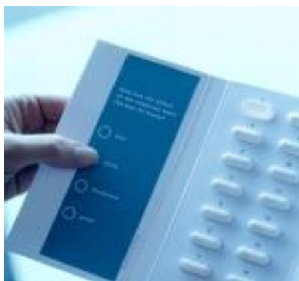
Fig.2: Removal of pills is tracked and the information can be sent to an electronic database
