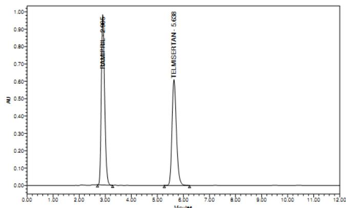
Figure 2: HPLC Chromatogram of Telmisartan and Ramipril.
