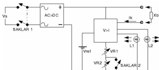
Figure 1 Diagram of Constant Current Iontophoresis Device
