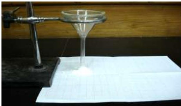
**Figure:** Measurement of angle of repose (Fixed Funnel method).
